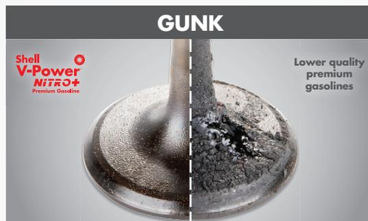
Intake valve deposit results based on a 10,000 mile vehicle fleet test of port fuel injected vehicles comparing Shell V-Power® NiTRO+ with lowest additive concentration (LAC) gasoline.
