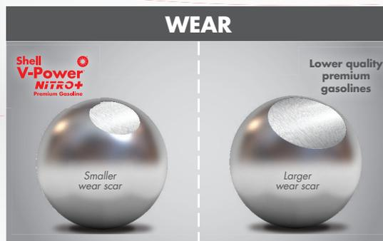
Wear results obtained using ASTM D6079 comparing Shell V-Power® NiTRO+ with lowest additive concentration (LAC) gasoline. Results depicted may not reflect what consumers see in their vehicles under normal driving conditions.
