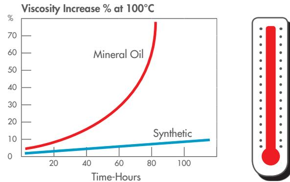
A comparable lubricant formulated with a synthetic base stock is inherently resistant to the oxidation reaction. This is because of the uniformity of the molecular structure and its engineered design that prevents the molecule from having any weak spots for the oxygen to attack. This resistance provides oxidation stability, preventing both sludge from forming and oil from thickening. More importantly, it can provide a longer drain interval and better wear performance.
