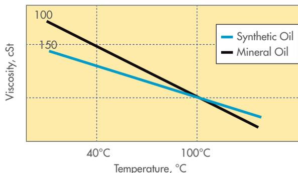
The synthetic base stock's inherent high viscosity index means a wider operating temperature range, better oil flow at cold temperatures, and thicker oil film at hot temperatures. Better lubrication across a wider temperature range means less wear and a longer component life.
