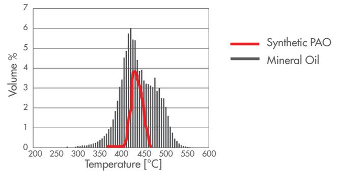
A synthetic lubricant has a tighter range of molecular structures and boiling points, causing it to be much less prone to volatilization. Using a fluid that will help reduce volatility in emissions is an easy fix from a cost standpoint. Even further, this is the solution of the future. More and more engines are going to be leaning towards these higher performing synthetic base oils.
