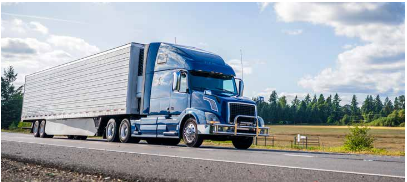
FIGURE 3. Tractor-trailer with chassis fairing and trailer skirt.
