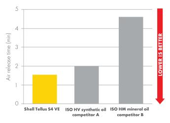
Air release test ASTM D34272
