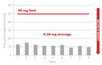
Bosch Rexroth RFT-APU-CL rig test
